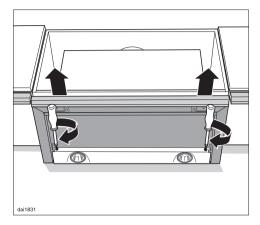
The position of the deflector plate can be brought forward by up to 35 mm using the adjusting screws on either side of the deflector plate. Align the deflector plate to the front of the kitchen furniture units on either side.
